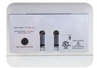
The table's electrical receptacles feature a new tool required access door designed to restrict unauthorized use of the outlets. Door easily unlocks so accessories can be plugged into the UL Listed, hospital grade receptacles. Once in place, the door closes over the electrical cords, securing plugs in place with the locking mechanism. Receptacles have a 9 amps total maximum load.
