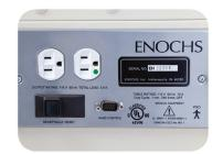
The hospital grade dual electrical outlets are conveniently located at the foot end of the table. The outlets feature a dedicated circuit breaker that will trip if outlets are overloaded. A quick reset of the circuit breaker re-establishes power to the outlets, eliminating costly down time. The Power 4250 also features a SELV (safety extra low voltage) hand control, an accessory that can be ordered at time of purchase or added at a later date.
