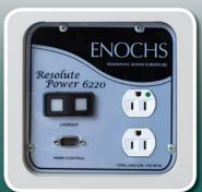
Quick access to electrical receptacles and the safety lockout switch on the side of the table saves time. The innovative Lockout System disables the hand and foot control to eliminate accidental table movement during exams or procedures but retains power to table's receptacles.
